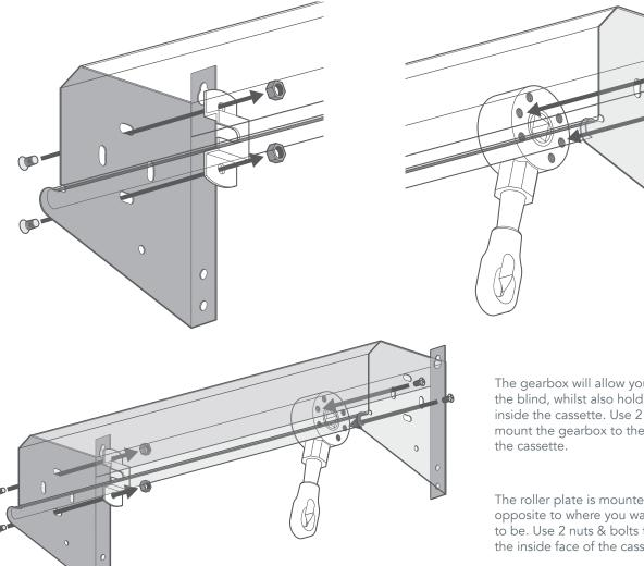
The gearbox will allow you to operate the blind, whilst also holding it in place inside the cassette. Use 2 screws to mount the gearbox to the inside face of
