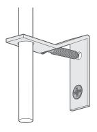
Feed the L-brackets onto the bottom of the side runners and fix them in place with 2 screws each.
