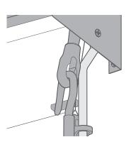
To raise or lower the blind simply rotate the crank handle.
