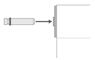
Start by inserting the roller 'pin' in the end of the blind opposite to the crank side. Note that the rubber 'O' ring on the pin should be resting inside the innermost of the two cutout sections.
