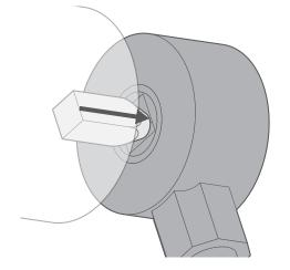
Now raise the blind up into the cassette and slot the square 'peg' on the crank side into the square slot in the crank.
