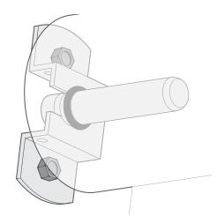
Raise the other end of the blind and slot the roller pin forward into the slot on the roller plate. Insert the R clip by pushing it up into the holes on the side of the roller plate.
