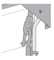
Feed the eyelets on the ends of the bottom bar up onto the ends of the side runners, then use the crank handle to raise the blind slightly.
