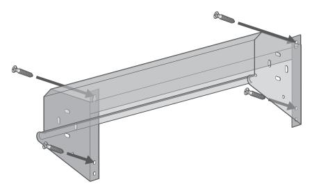
Use 4 screws to mount the cassette to the wall above the window. The cassette will be the 'cover' for the bind.
