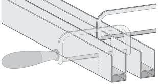
Use a fine-tooth saw to neatly cut through each channel where you made your marks.
