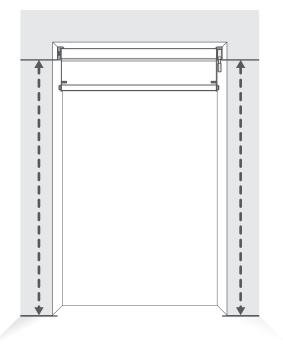
The side channels are provided to you longer than the drop you ordered, so that they can be trimmed to the perfect length. Measure for this by measuring up from the ground to the lowest edge of the brackets.
