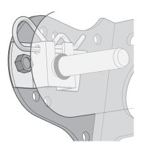
Secure the blind by slotting the R pin through the roller plate.
