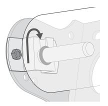
Slot the roller pin into the end of the roller, then raise that end and drop the groove of the roller pin into the cutout in the roller plate.
