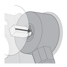
Lift the blind to the brackets and slot the square peg on one end of the blind into the corresponding hole in the gearbox.
