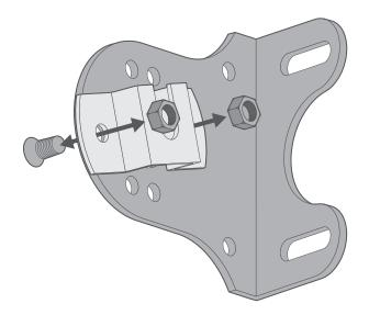
Start by fixing the roller plate to the bracket opposite to the control end. Use 2x nuts & bolts to attach the plate to the inside face of the bracket.
