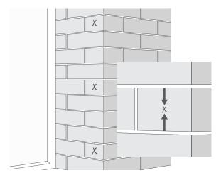
When you install the side channels you should really try to make sure you're screwing them into brick, not into the mortar between the bricks.
