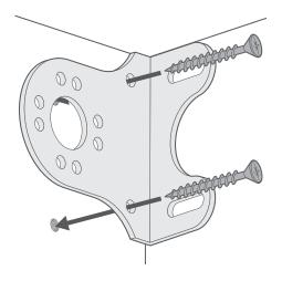
Use 2x screws and plugs per bracket, to side-fix the brackets to the inside face of the recess.
