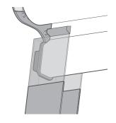
Take the side channels and feed the caps on the blind's bottom bar into the tops of the channels. Hold the channels in position and check them with a spirit level to make sure everything's straight.
