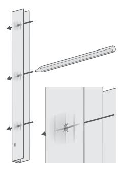
Use a pen or pencil to mark out where the screw holes will go - in theory these marks should line up with the marks you made on the wall originally, but it's best to do this again as you'll likely find after checking with your spirit level that the positions of the screw holes are a little different.
