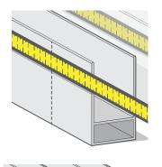
Mark the measurements out on the side channels, being sure to mark the correct channel with each.
