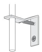
Feed the L-brackets onto the bottom of the side guides and fix them in place with 2 screws each.
