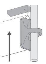
Feed the eyelets on the ends of the bottom bar up onto the ends of the side guides, then use the remote to raise the blind slightly.
