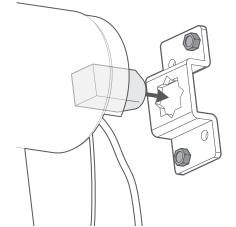
Now raise the blind up into the cassette and slot the square 'peg' on the motor side into the star-shaped slot in the roller plate.
