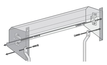
Use 4 screws to mount the cassette to the inside walls of the recess. The cassette will be the 'cover' for the bind.
