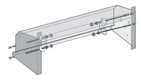
Mount the roller plates to the inside of the cassette, as shown. Use 2 nuts and bolts per plate.
