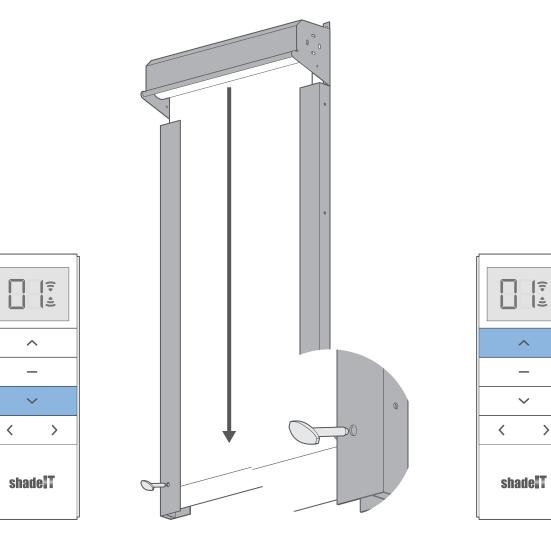
Use the remote to lower the blind. Allow it to lower until it reaches the lower limit point you set before. Insert the plugs into the bottom of the side channels.
