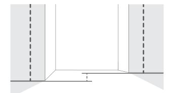
Make sure you measure each side separately, as the ground may be uneven, making one side higher then the other. Make a note of each length measurement.
