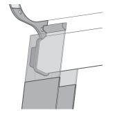
Take the side channels and feed the caps on the blind's bottom bar into the tops of the channels. Hold the channels in position and check them with a spirit level to make sure everything's straight.
