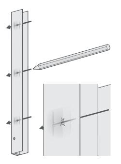
Use a pen or pencil to mark out where the screw holes will go - in theory these marks should line up with the marks you made on the wall originally, but it's best to do this again as you'll likely find after checking with your spirit level that the positions of the screw holes are a little different.
