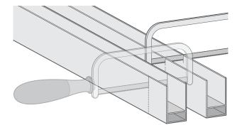
Use a fine-tooth saw to neatly cut through each channel where you made your marks.
