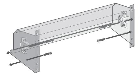
Use 4 screws to mount the cassette to the inside walls of the recess. The cassette will be the 'cover' for the bind.
