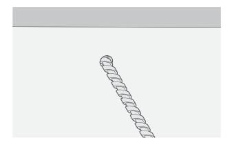
Drill holes into the lintel where you marked out the holes for your brackets, and insert a rawl plug into each hole.
